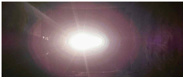
Image 1. Light from both flashlights with no smoke in the box. The light output at 8 feet was measured at 172 Lux for the Maglite and 1.92 Lux for the Nightstar.
