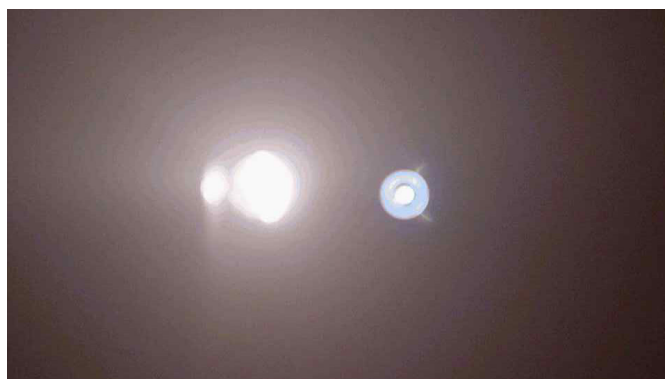
Image 3. Light from both flashlights after some of the smoke was removed from the box. The light output from the Maglite was measured at 3.61 Lux and the output from the Nightstar was 0.16 Lux.
